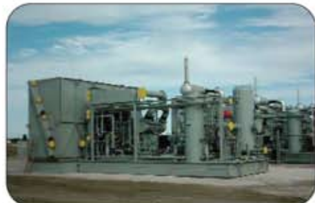
Each hour that a compressor like this one is down can cost an operator thousands of dollars in lost production. Implementing remote compression monitoring at one field site can result in a reduction in downtime of up to 25 percent.
